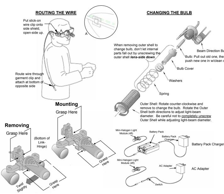
DO NOT grab or misalign telescope oculars! DO NOT pull or push the outer shell!
